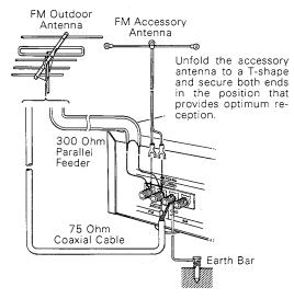
**CAUTION:** Never make a connection to a gas pipe because it can cause fire hazard.
