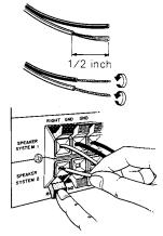
**CAUTION**: Two speaker systems can be connected to this unit. The minimum speaker impedance should be 8 Ohm when only one speaker system is connected. When two speaker systems are connected, care should be taken that net impedance does not become less than 8 Ohm.
